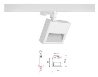
17W LED Triac dimmable commercial wall washer track fitting with neat and clean bracket features a no visible wire aesthetic. 355° rotate and 90° tilt makes it a great general purpose light. Produces a wide, uniform square shape light, useful for washing Description:
