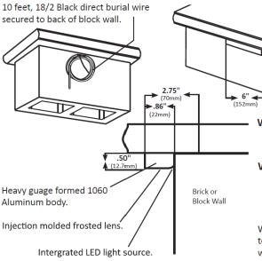
Locate fixture in the hardscape. Test fixture placement and spacing before adding mortar and installing the cap.
