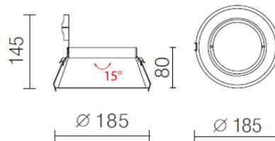
**Description:** Extra thin trim floor/wall washer downlight compatible with GU10, Mr16 or module. IP44, perfect for high end bathroom and commercial settings. Lamp replacement via front ring for easy maintenance.
