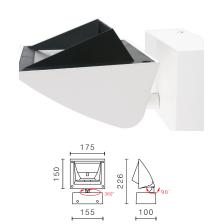
25 watt COB LED interior wall mounted luminaire providing wide wall and ceiling washing effect. Purpose made optical reflector provides a square uniform light output. Special baffle frame offers superior glare control. No UV/IR radiation. Description:
