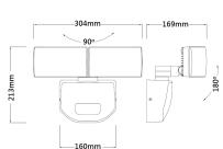
Description: 25W Sensor light with durable ABS polycarb construction. UV & corrosion resistant. Inuilt microwave sensor, with dip switch
