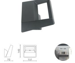
Description: IP65 Square module LED light head, can be installed as door (wall) light. Die-cast aluminium body with LED technology providing long life time at low maintenance cost. Inbuilt driver included, and easy to install. Anti-dazzle shielded light head with asymmetric light distribution. Creates soft and trendy visual effect on the wall. Colour temperature adjustable.
