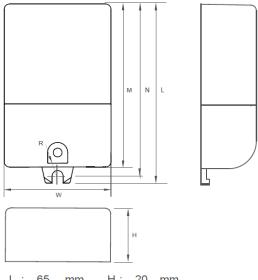
L: 65 mm H: 20 mm M: 59.2 mm R: 2 mm N: 62.5 mm W: 39 mm
