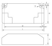
85 L: mm W: 40.4 mm H: 22 mm M : 76.4 mm **K**: 4.0 mm N: 4.6 mm
