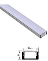
Description:2.5 metre slimline surface mount extrusion with opaque diffuser. LED strip light not included. Optional clips & end caps available.Material:Aluminium Alloy, PolycarbonateLens:Opal Diffuser as standard. Optional clear diffuser, UV rated diffuser or black diffuser available on request.Mounting Type:Surface Mount
