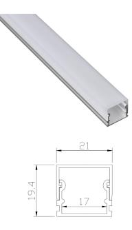
Description: 21 X 19.4 Surface mount extrusion suitable for taking strips of up to 15mm PCB width. Diffuser is wrap around U-shape so will have a wider beam angle compared to our standard slim (BARSMPU-F) and deep (BARSMPU-2D) diffused extrusions. Black or white extrusions are available on request, please enquire for quotation.
